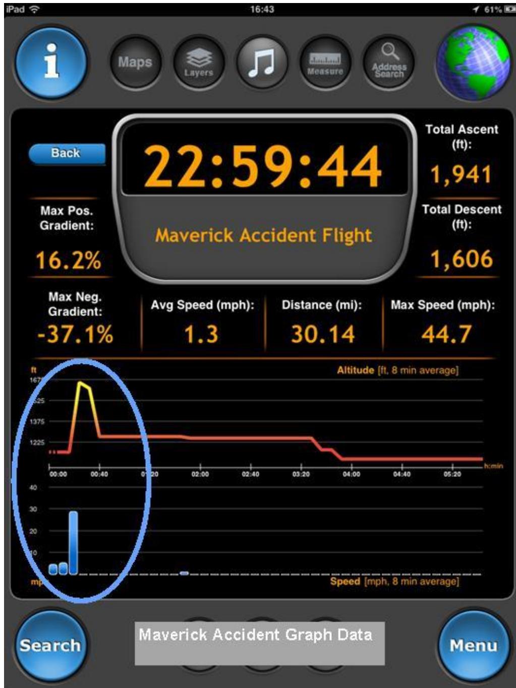
Picture 027 Performance data of flight. Flight data continued to record after initial flight and accident. Flight data totals include an additional 22 1/2hrs of recording post crash movement including transport of Maverick from scene of impact.
