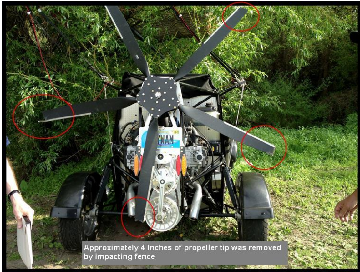
Picture 022 Propeller Tips separated by contact with fence
