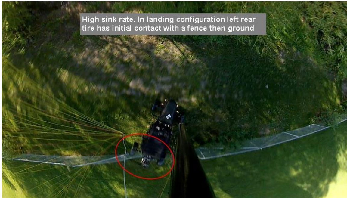
Picture 019 At a high sink rate but in a landing configuration, aircraft impacts fence with rear left tire
