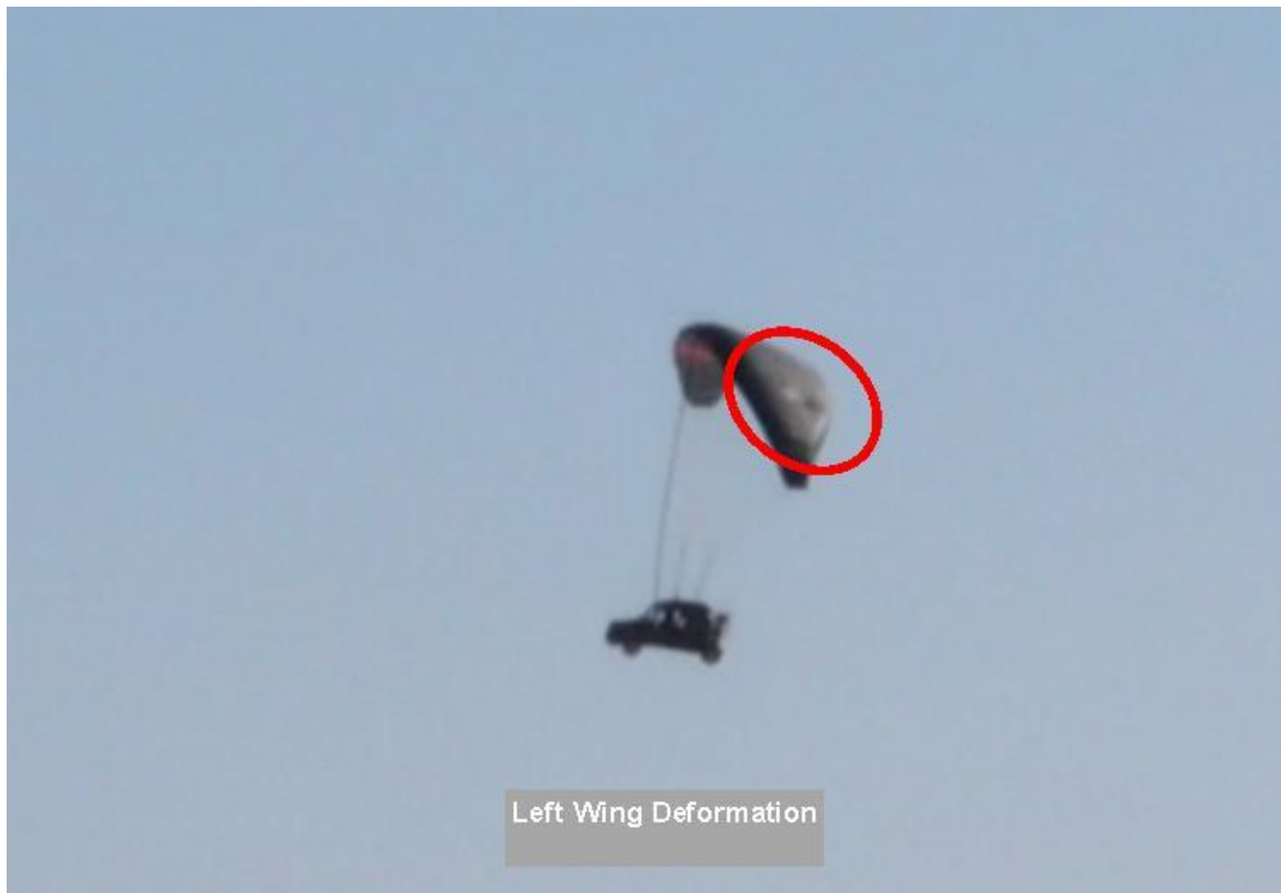
Picture 009 Dimple in left wing indicates how severe the wing deformation was
