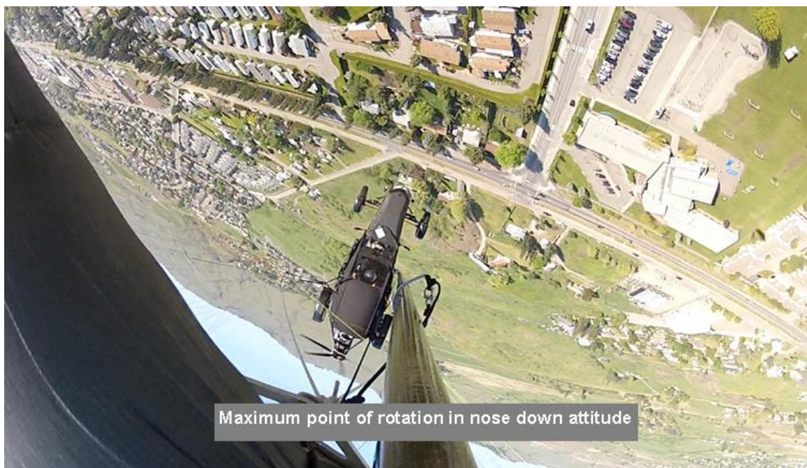
Picture 015 Stall / Spin developed quickly and immediate full power and opposite controls were applied even before full development was complete.
