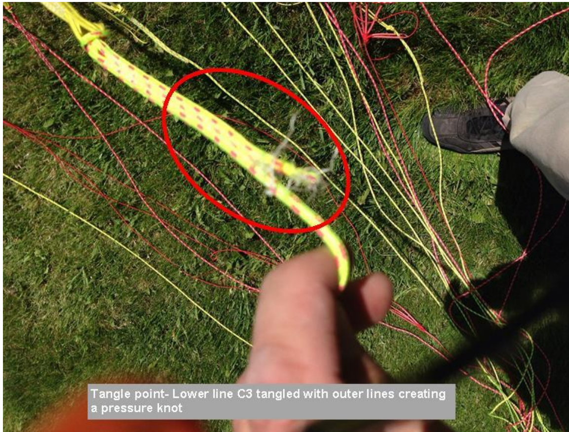
Picture 008 Post accident line analysis shows tangle point
