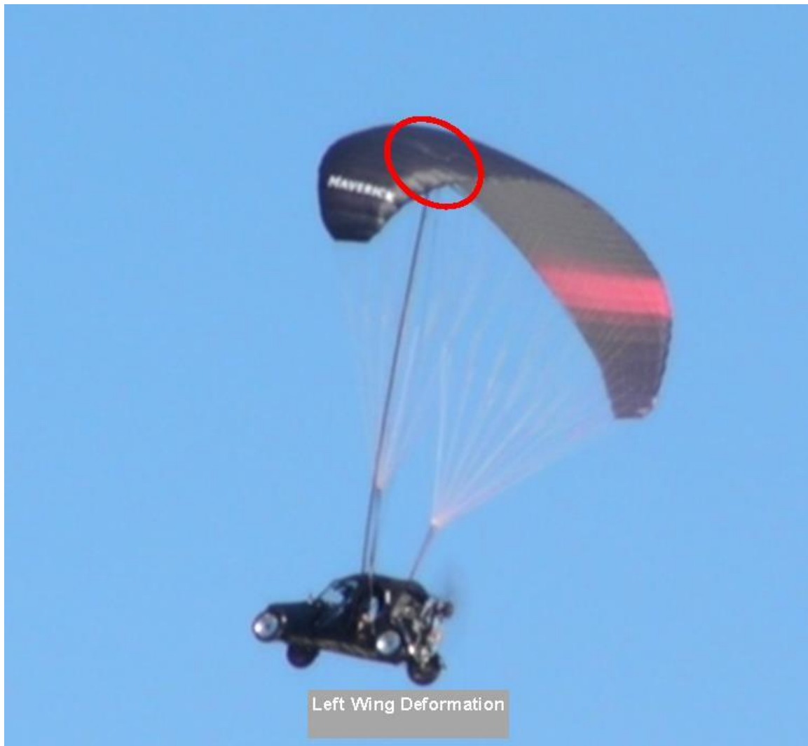
Picture 010 Left wing deformation closer view
