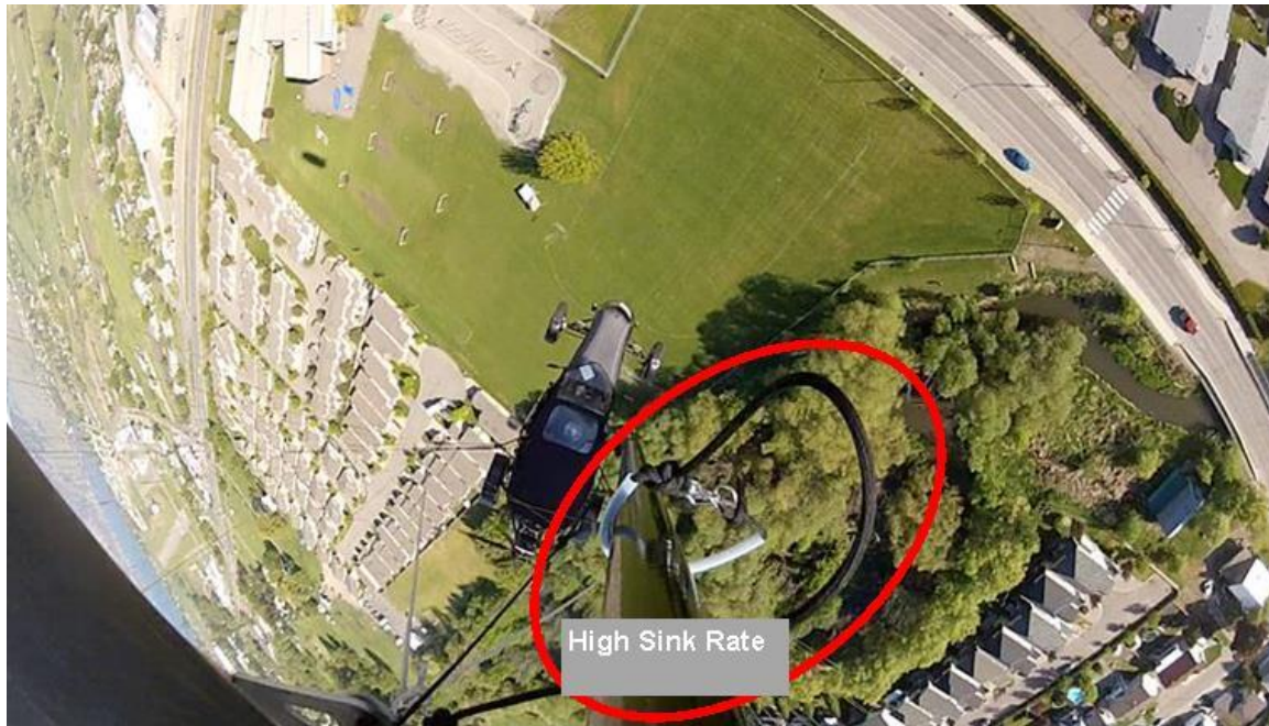
Picture 017 Retaining ring floating up illustrates the high sink rate experienced
