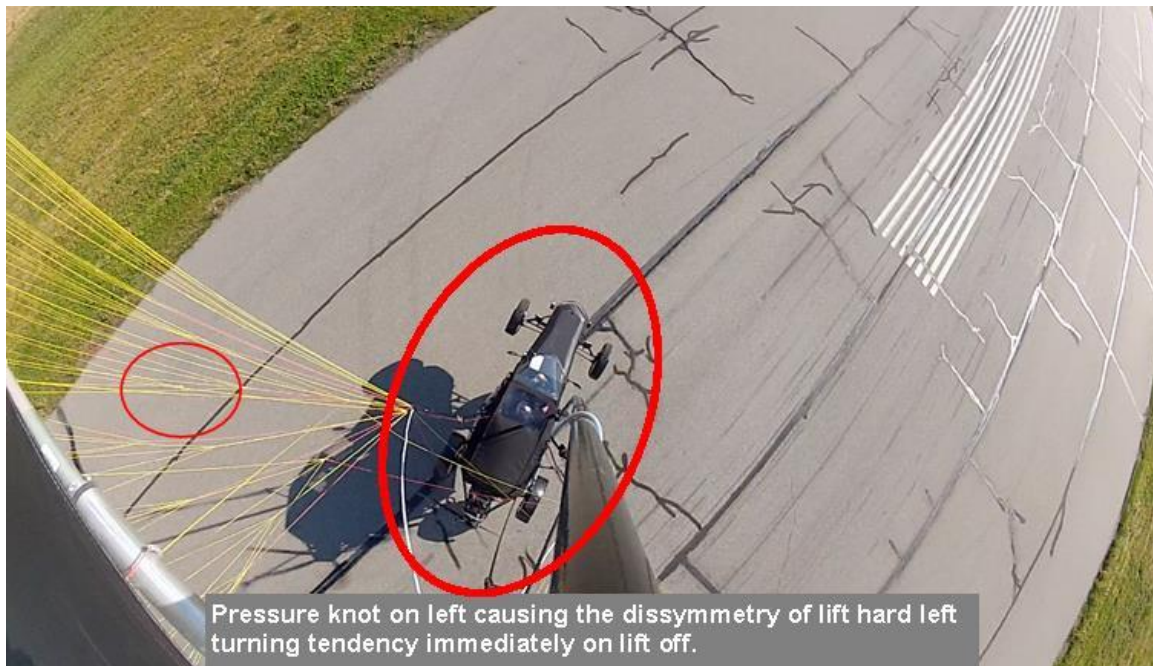
Picture 012 Initial take off and immediate left turning tendency
