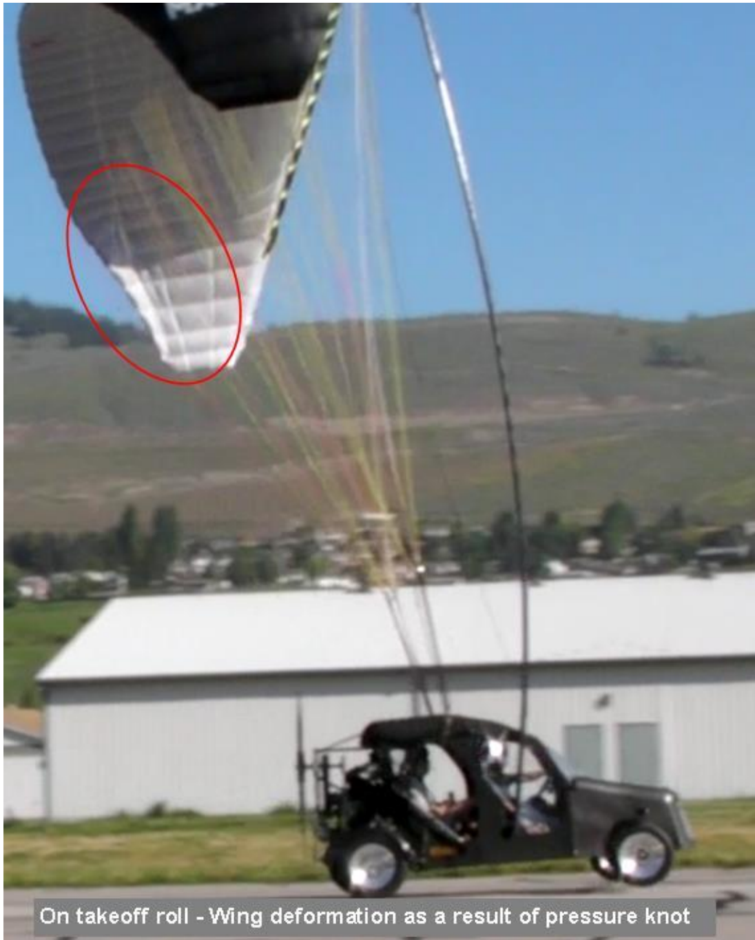
Picture 007 Wing Deformation Side view
